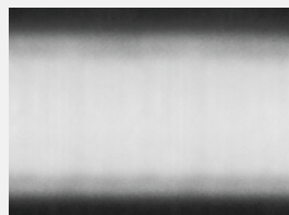
Latex emulsion paint through a HEA 517 tip at 1,000 PSI
